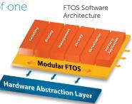
FTOS leverages a distributed, multiprocessor architecture that delivers highly scalable protocols and reliability in each product line. Z-Series and E-Series Route Processor Modules (RPMs) are designed with separate control plane CPUs for Layer 2, Layer 3 and management functions, with distributed processing on line card CPUs. The C-Series RPMs and S-Series switch/routers use one control plane CPU, with distributed processing on C-Series line cards and S-Series stack members.
